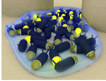
Fig. 1. Concept of a robotic system built of swarmer and a passive membrane, changing its shape to get through the gap in the background
